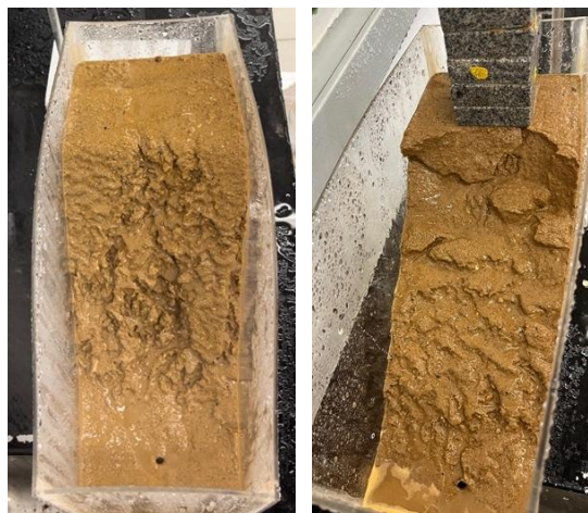
Figure 5 – Failure mechanisms of surface erosion (a) and rotational landslides (b)
